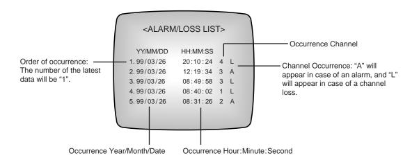
Once the alarm is on, you can check the time the alarm went on along with the relevant channel. This information remains in nonvolatile memory so you can check the information even after the system has been powered off.
